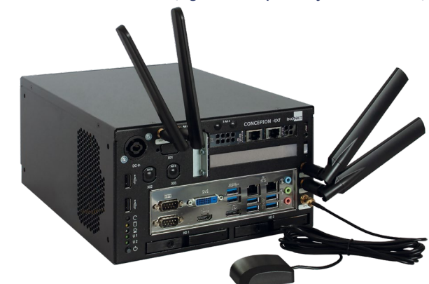
Wi-Fi/Bluetooth and GNSS/LTE (optional) (Fig. without QuickTray®-v3 extension)
