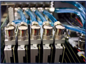
Up to 5x Tensor cards PCIe x16/x8 Liquid cooled
